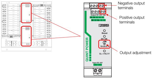
The power supply shown is a DC/DC, however the terminals and adjustment potentiometer are located in the same place on an AC/DC power supply
