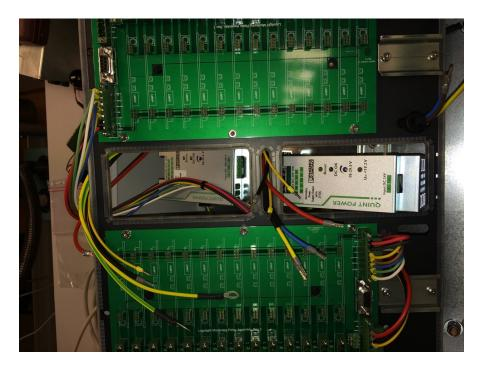
Change the faulty Power-supply unit (remove by releasing DIN-rail bracket under the power-supply unit
